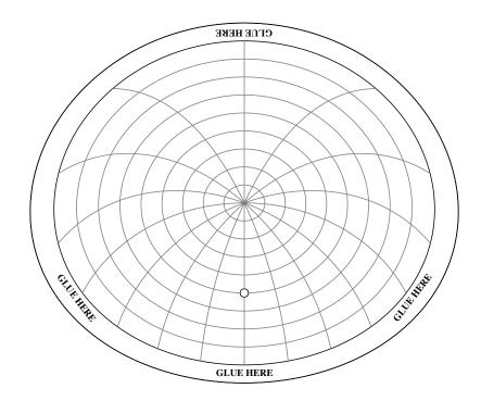
This grid of lines can optionally be printed onto transparent plastic and glued into the cut out window in the planisphere's body to show the altitudes of objects in the sky, and their directions.
